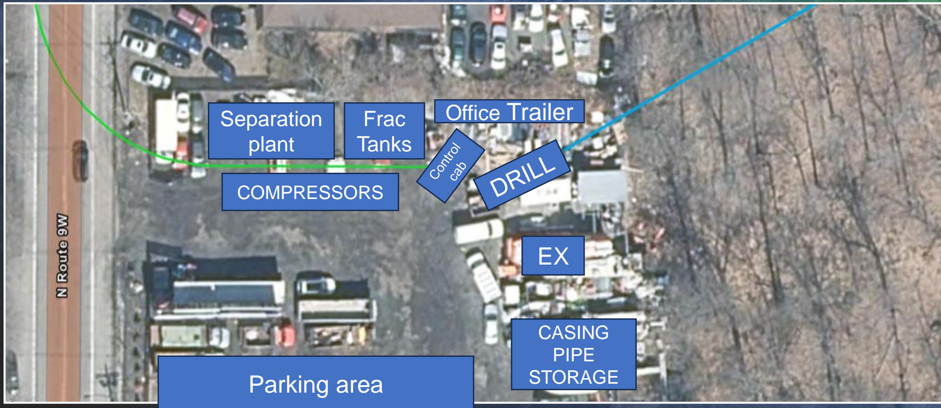
Congers NY Site aerial with equipment layout and bore path
