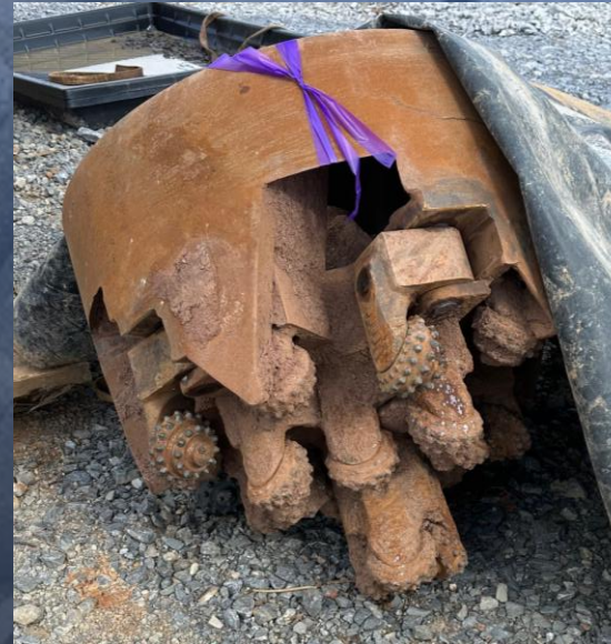
Various auger Boring cutting heads L. Disc Cutter C. Christmas Tree R. Roller-Cones
