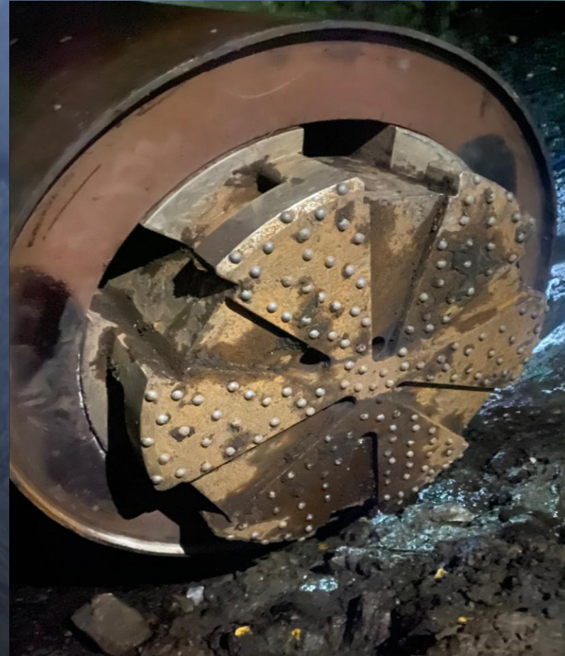
Pilot Bit protruding through start casing. Intermediate Shoulder resting on internal Collar of start casing.
