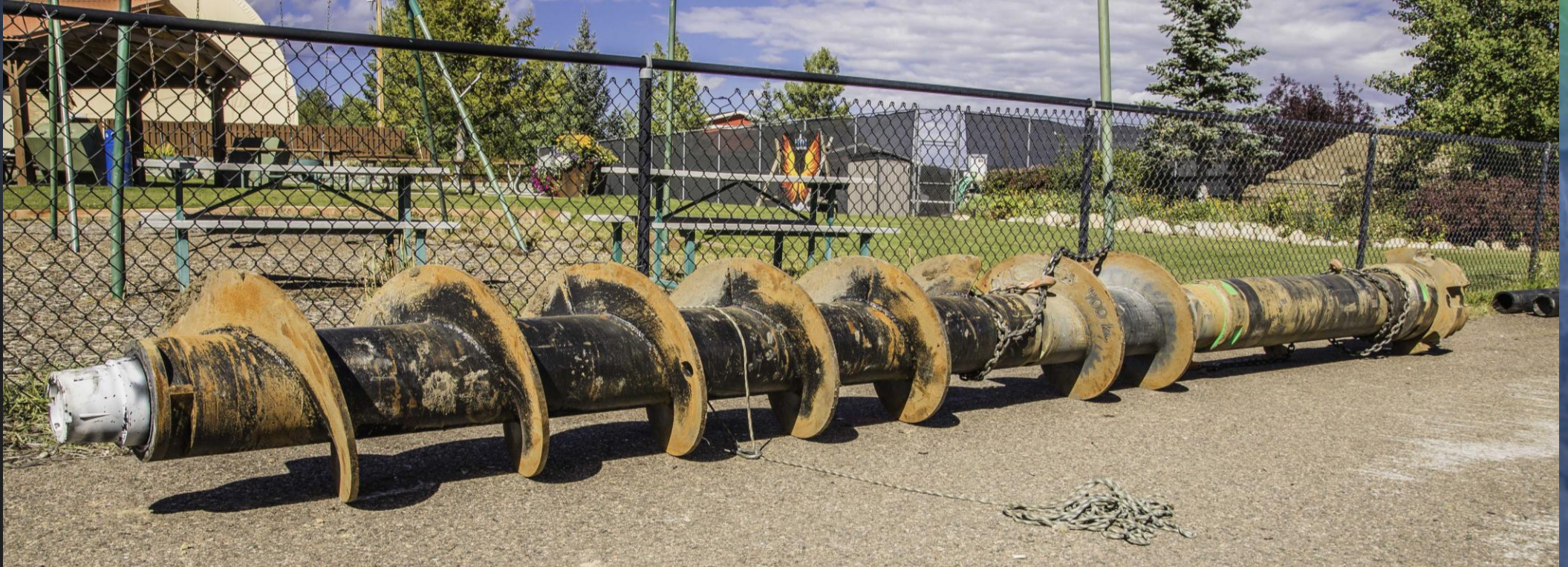
Down-Hole Tooling Left to Right: Auger – Hammer – Pilot Bit
