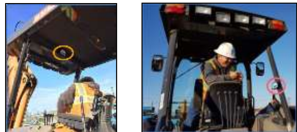
Figure 2: Device installation locations
