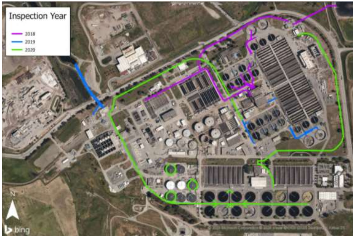
Figure 2: Yard Piping Assessed to Date
