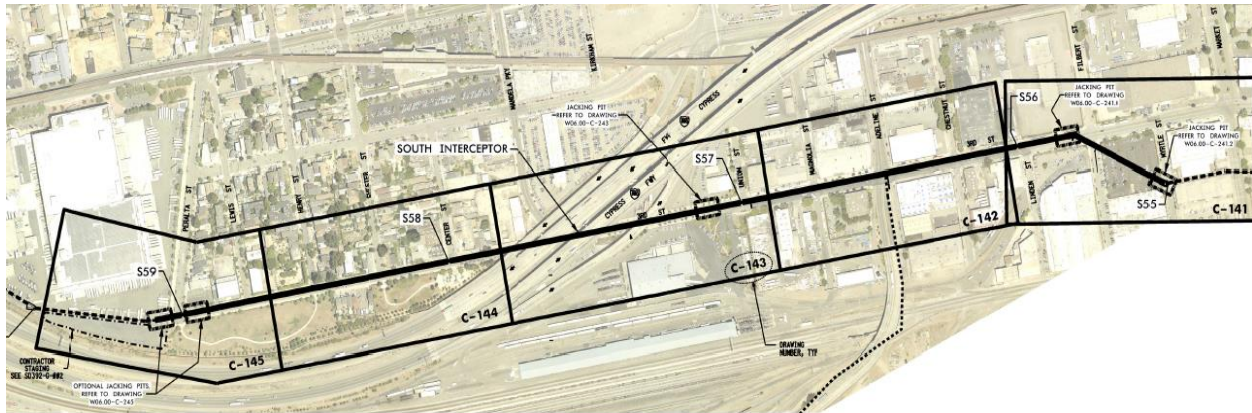
Figure 4. Locations of the five planned sliplining pits
