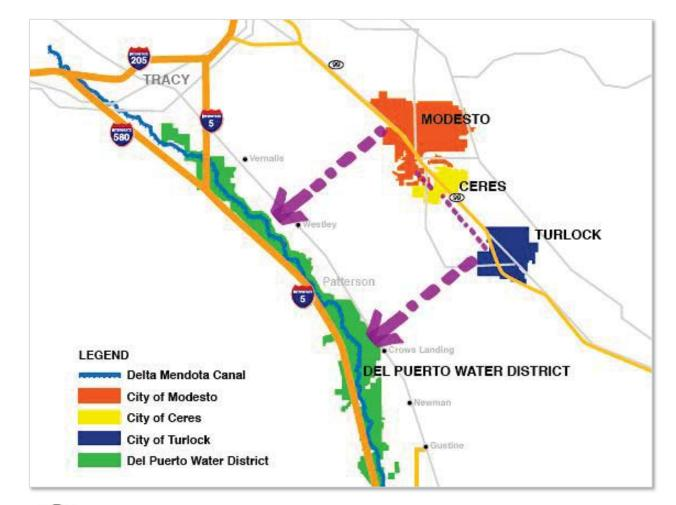
**PROJECT BACKGROUND** Recycled water will be conveyed to Del **Puerto Water** District via a pipeline from the **Cities of Modesto** and Turlock to the **Delta-Mendota Canal**
