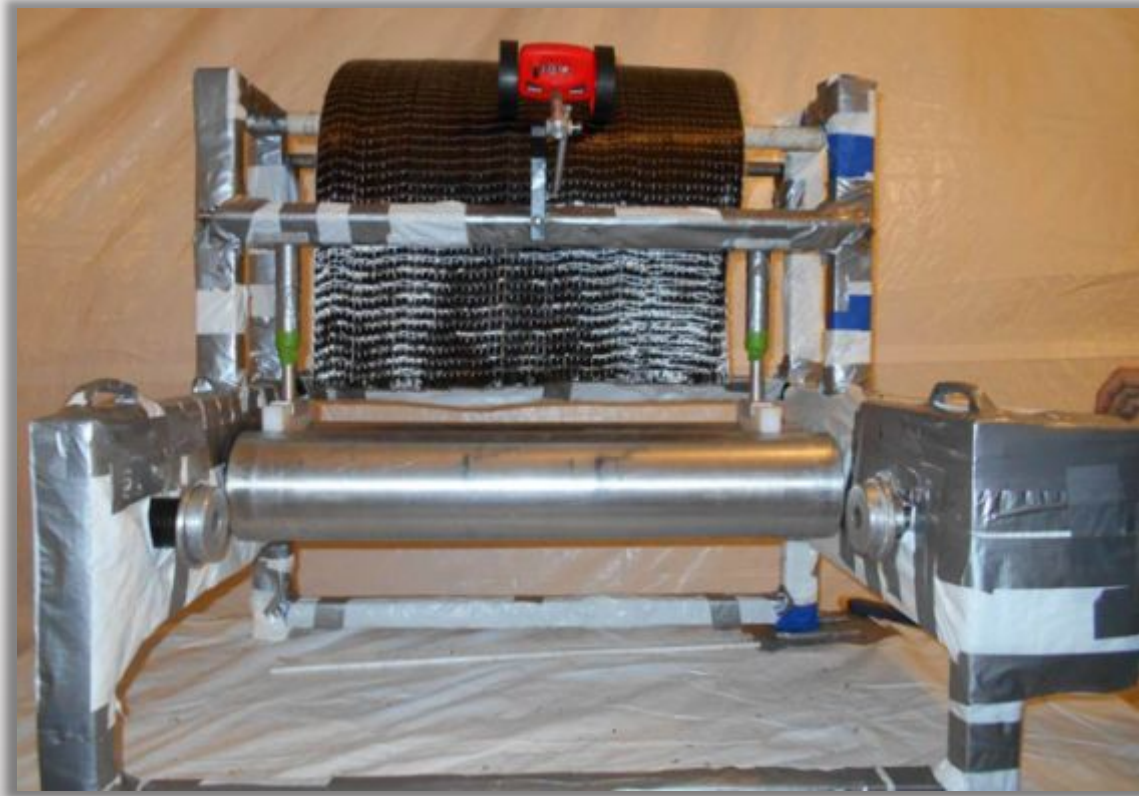
Mechanical saturator for CFRP
