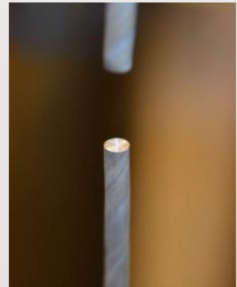
Torsion fracture surface of uncorroded wire
