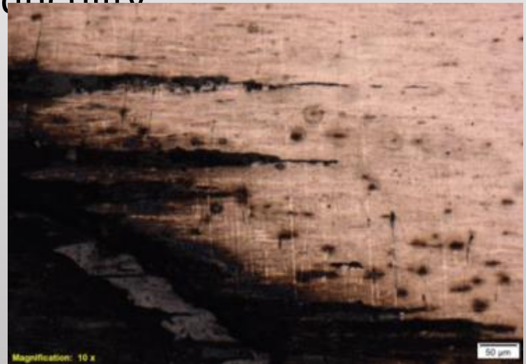
Longitudinal splits and corrosion oriented along the wire axis
