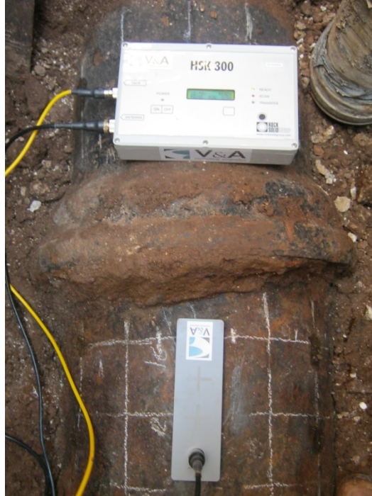
Photo 1. BEM Antennae and Electronic Console
