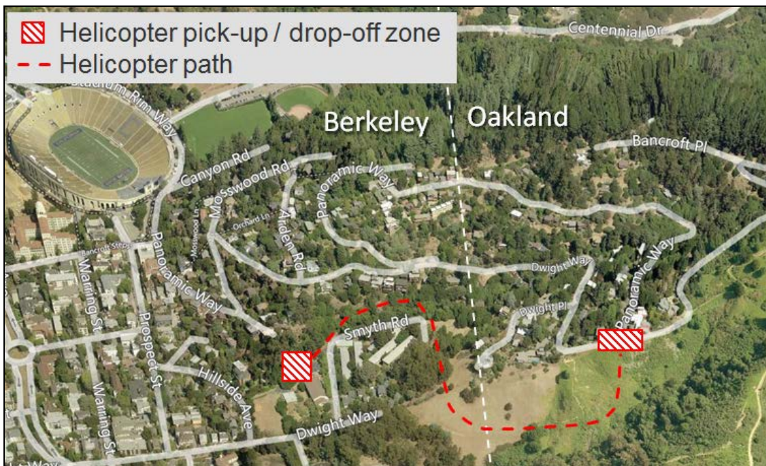
Figure 3. Helicopter Flight Path for Delivering Pipe to the Panoramic Hill Pipeline Replacement Project
