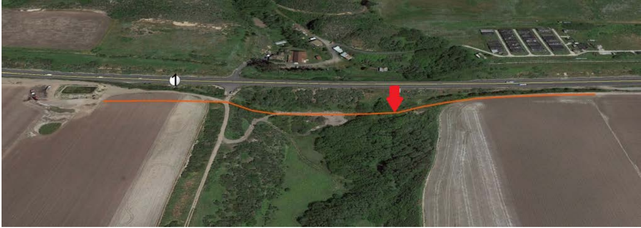
Figure 2: Lombardi Gulch HDD alignment in context with location of failure in parallel existing main.
